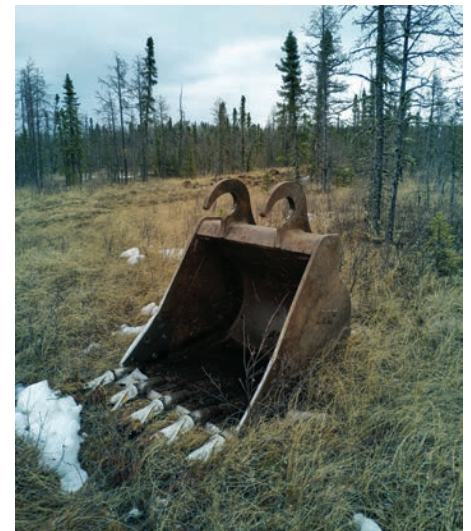
Figure 2B. A digging bucket (1 yard) equipped with frost-teeth.
