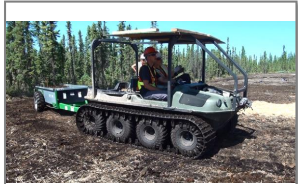
Figure 1: Moss Spreader attached to an Argo
