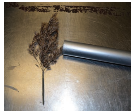
Figure 6. Vacuum nozzle (right) used to extract pappus from the stem.
