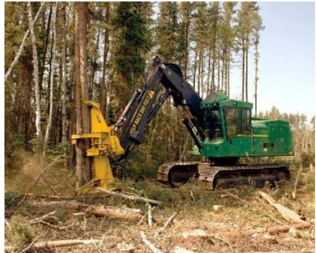
Figure 13. Feller-buncher harvesting trees.
