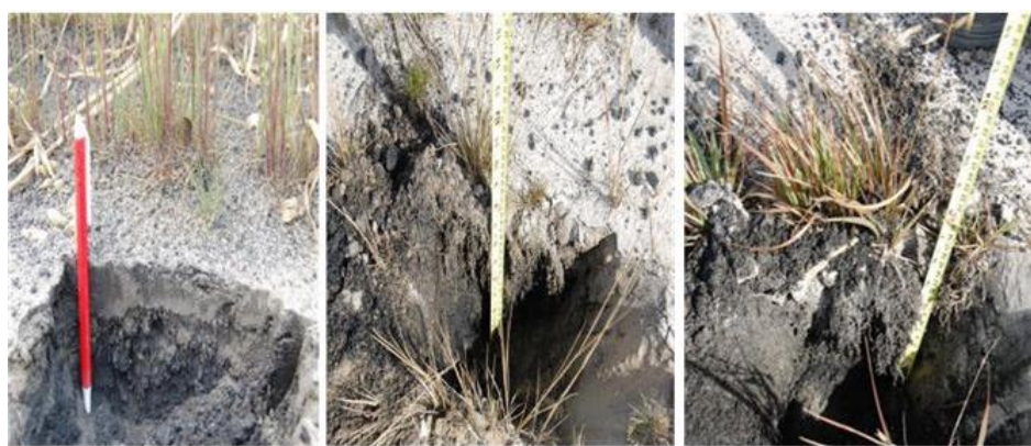
Figure 4 Growth of native grasses showing healthy roots not restricted by the coke layer in the shallow end (0–30 cm) of the tailings sand placement on the plots
