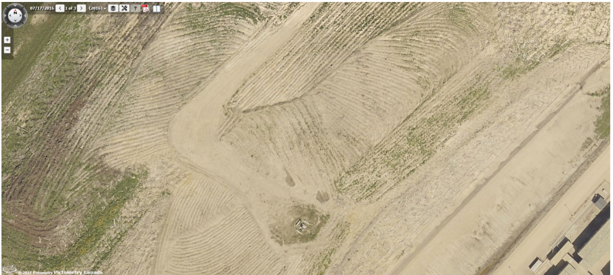
Figure B-12 Rough and loose site preparation and coarse woody material application completed fall of 2015. Vegetation trials planted June 2016 (image taken July 17, 2016).
