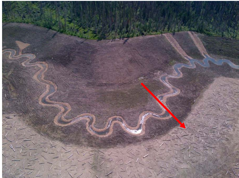
Figure B-42 Coarse woody material placed along the outlet channel at the compensation lake.
