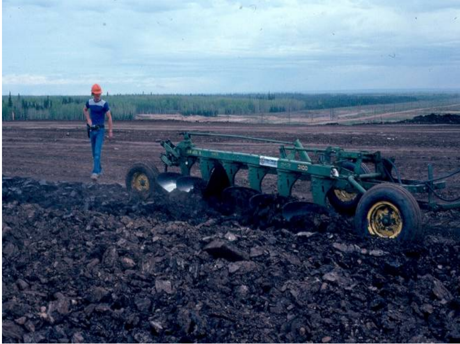
Plate 2.9. Mouldboard plow used to alleviate compaction at Syncrude Canada Ltd.
