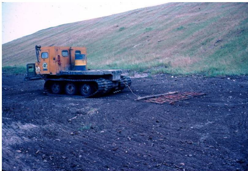
Plate 2.8. Harrows being pulled by an All Terrain Vehicle after seeding at Suncor Energy Inc.
