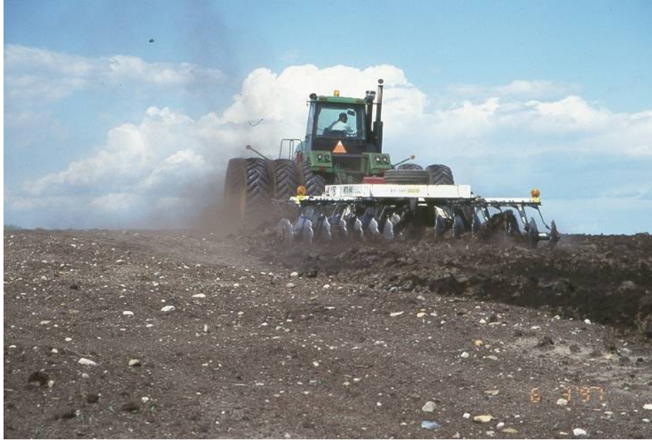
Plate 2.18. Disc incorporating peat mix into underlying secondary material at Syncrude Canada Ltd.
