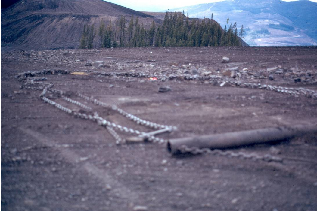
Plate 3.16. Chain drag used for surface scarification.
