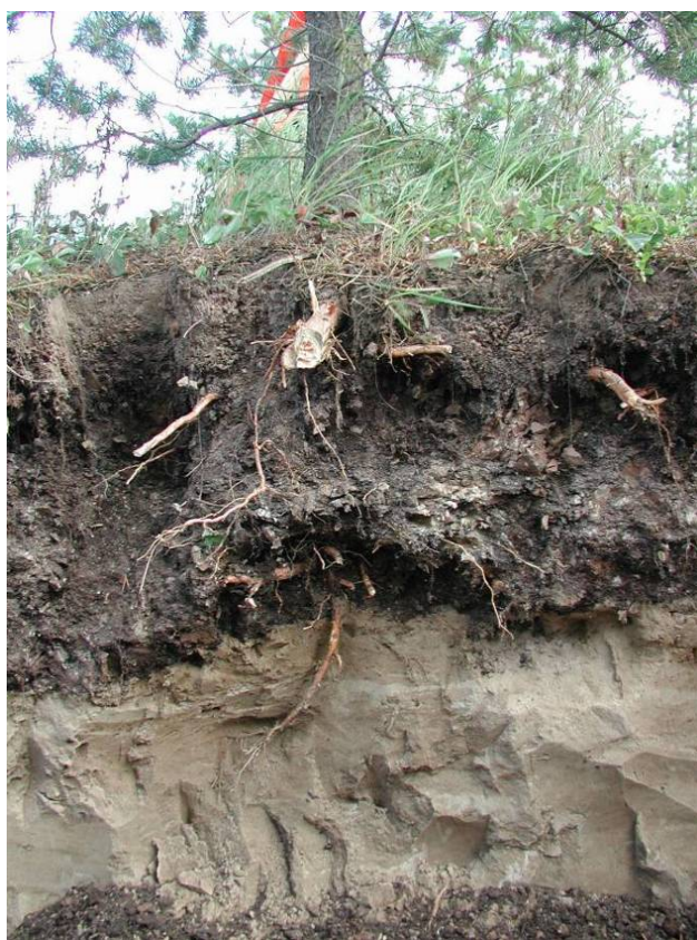
Plate 2.26. Root distribution in peat mix over tailings sand at Syncrude Canada Ltd.
