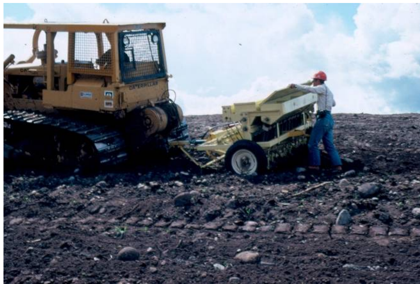
Plate 2.31. Drill seeder at Syncrude Canada Ltd.
