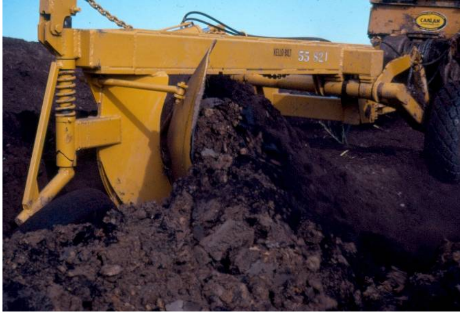
Plate 2.11. Kello-Bilt deep plow used for contour plowing in the 1980s at Syncrude Canada Ltd.
