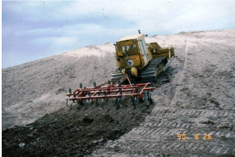
Plate 2.7. Chisel plow used At Suncor Energy Inc. after 1979.
