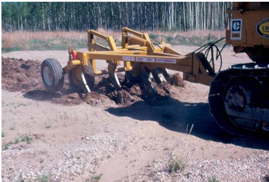
Plate 2.42. Kello-built deep tillage subsoiler at Syncrude Canada Ltd.
