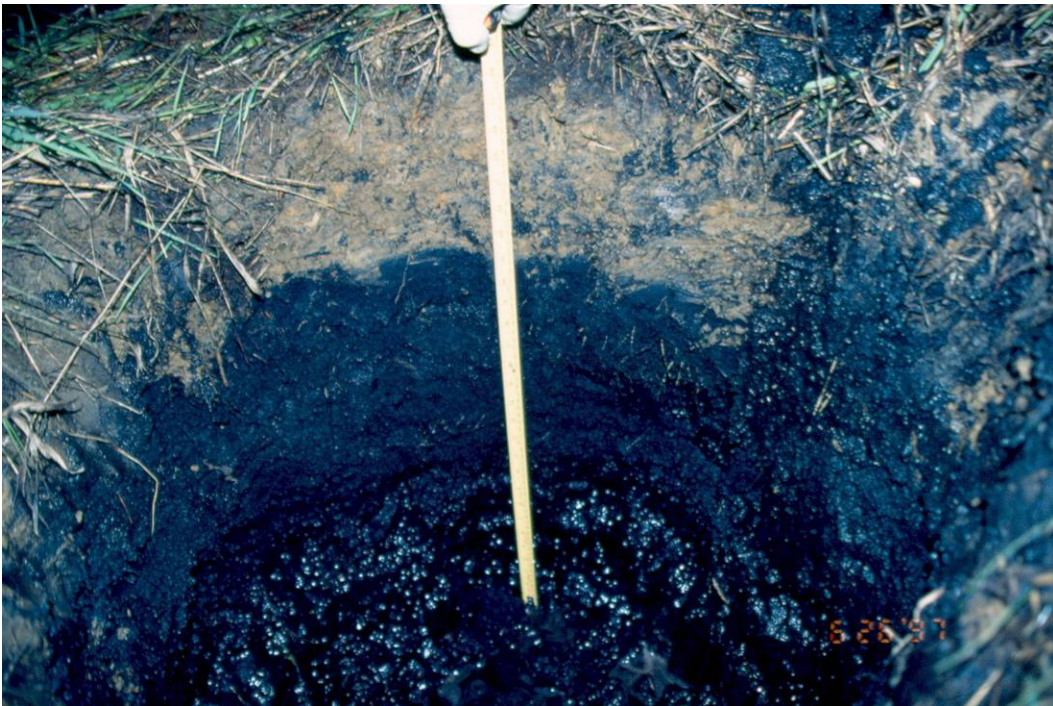
Plate 3.95. Soil cap over tailings.
