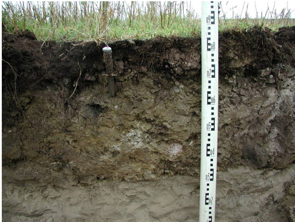
Plate 1.7. Peat mix tilled into secondary layer over tailings sand.
