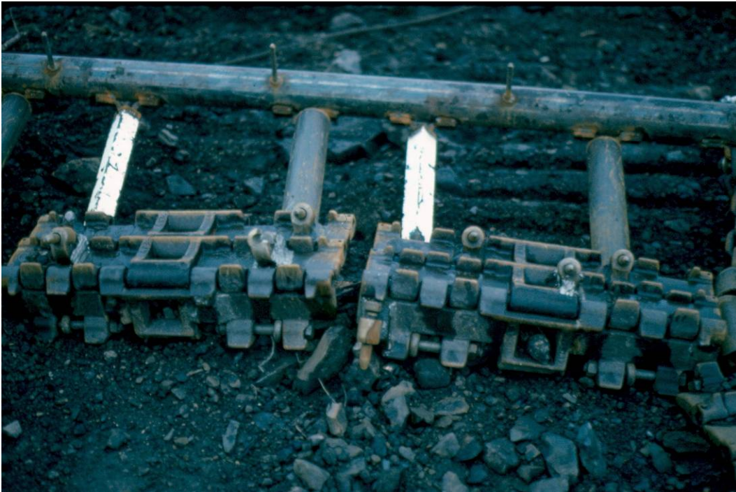
Plate 3.17. Drag comprised of independent sections.
