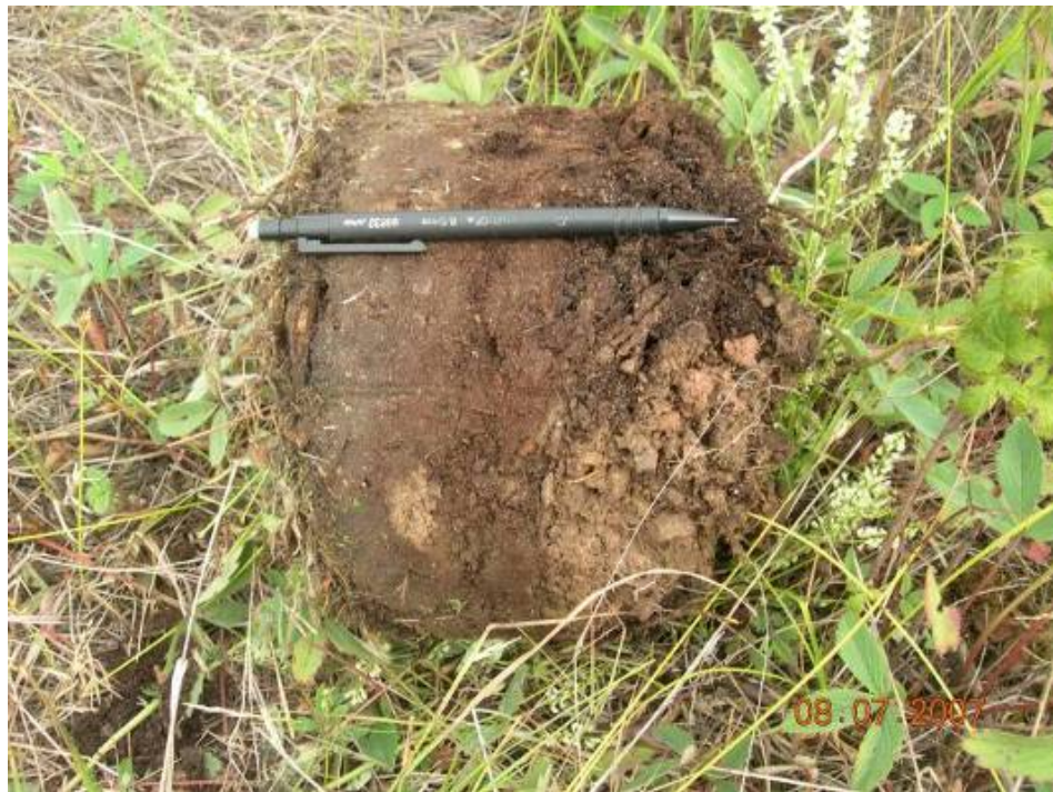
Plate 2.21. Cross section of replaced LFH layer at Syncrude Canada Ltd.
