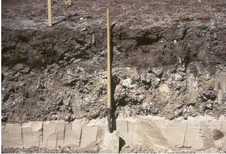
Plate 2.16. Cross Section of peat mix over secondary over tailings sand at Syncrude Canada Ltd.
