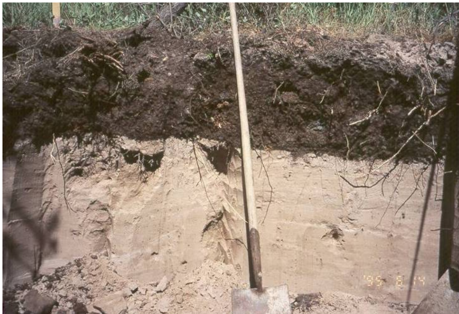
Plate 2.17. Cross section of peat mix over tailings sand at Syncrude Canada Ltd.
