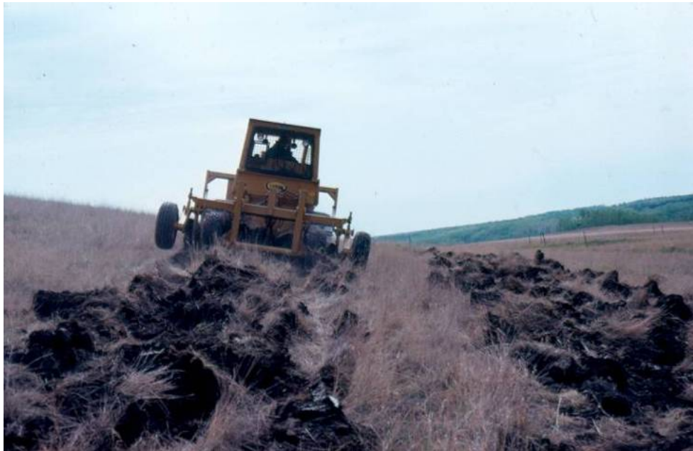
Plate 2.43. Soil surface after deep tillage at Syncrude Canada Ltd.
