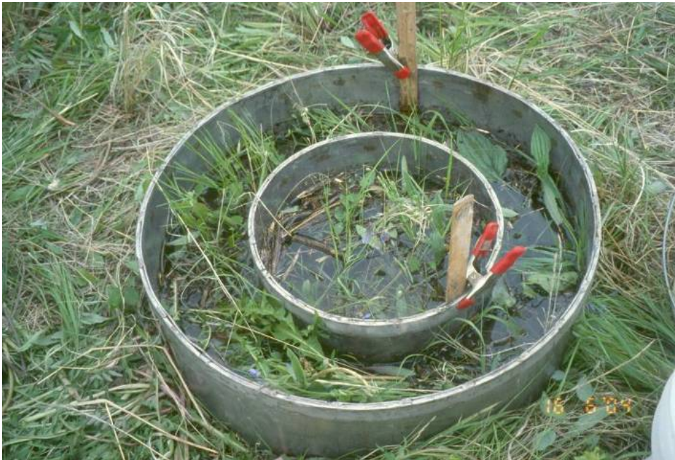
Plate 2.24. Infiltration measurement at Syncrude Canada Ltd.
