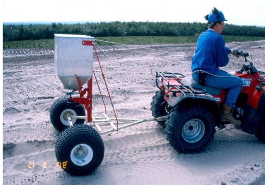
Plate 2.30. ATV seed broadcaster at Suncor Energy Inc.
