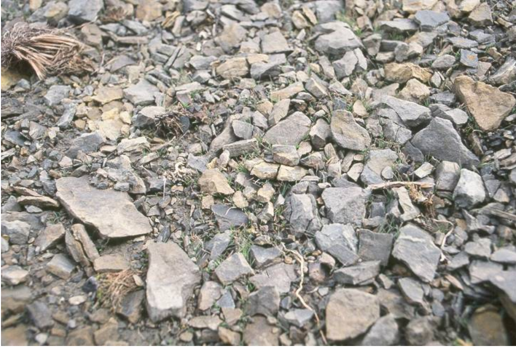
Plate 3.24. Rock spoil material as surface “soil” at No. 12 Mine.
