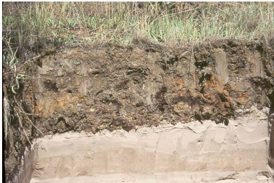
Plate 2.15. Cross section of secondary material over tailings sand at Syncrude Canada Ltd.
