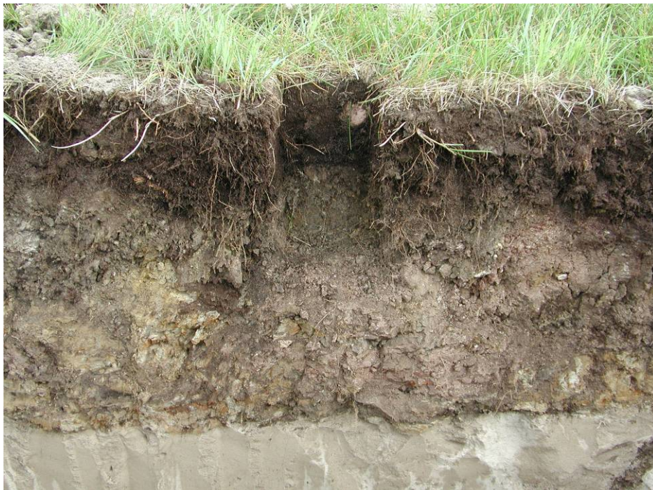
Plate 1.4. Peat-mineral mix over secondary over tailings sand.
