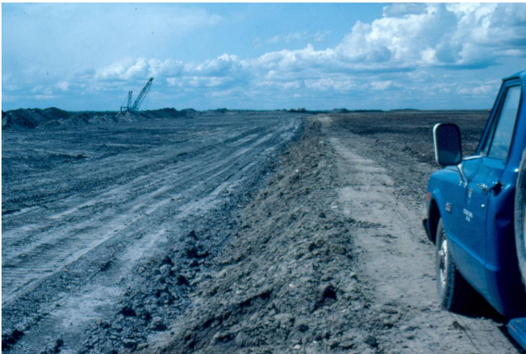
Plate 4.6. Topsoil, subsoil, spoil sequence at Vesta Mine.
