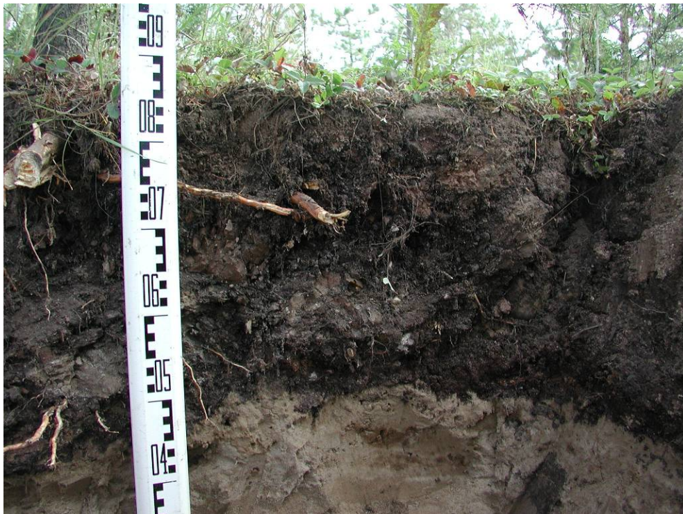
Plate 1.6. 40 to 50 cm peat-mix over tailings sand.
