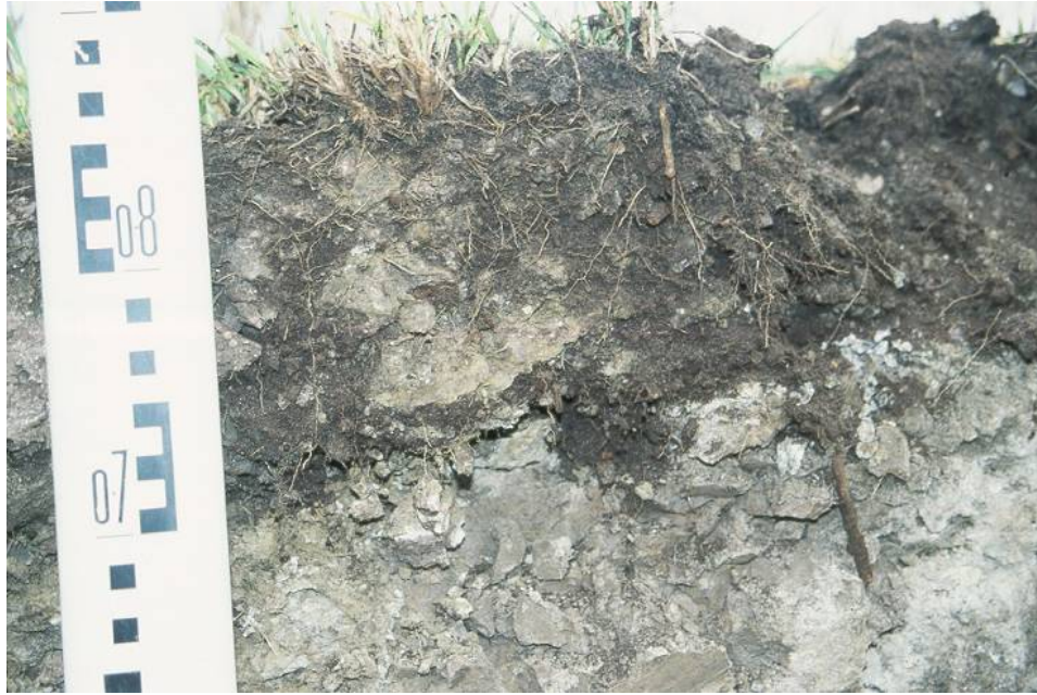
Plate 2.20. Peat mix and secondary over secondary material at Syncrude Canada Ltd.
