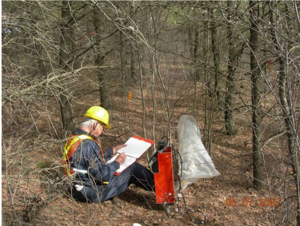
Plate 2.23. Soil moisture and density measurement at Syncrude Canada Ltd.
