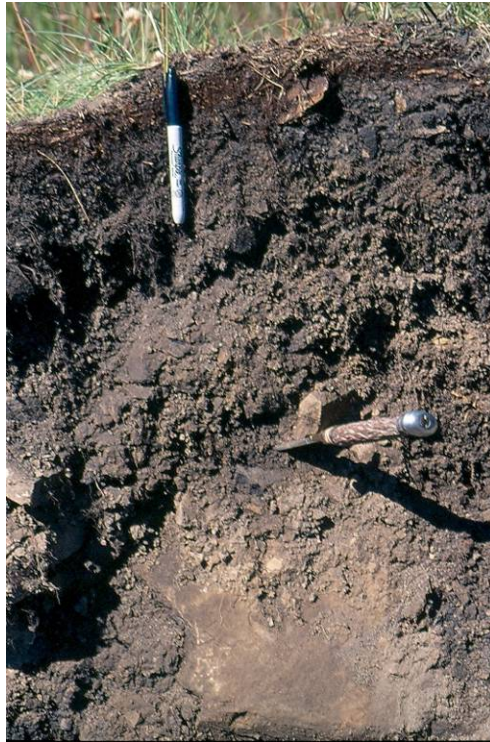
Plate 3.20. Cross-section of a reconstructed soil in 2005 (coversoil replaced in 1972).
