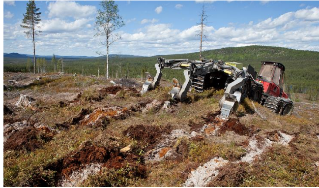
Figure 11. Examples of tow-behind-implements used in forestry to create microsites. Source: www.brackeforest.com .
