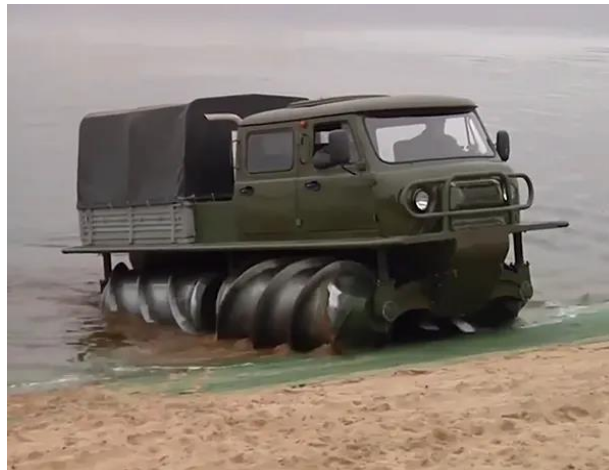
Figure 12. An example of a Russian screw-propelled vehicle. Source: Youtube/Ruptly https://youtu.be/nVOaDfGOPGs .
