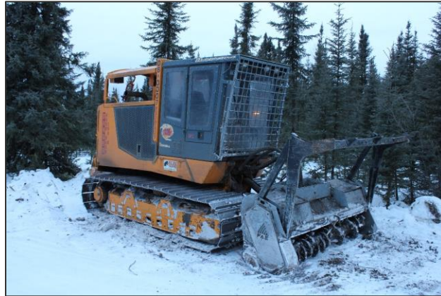
Figure 1. An example of a mulcher used to clear recent seismic lines in the boreal forest.
