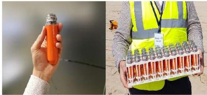
Figure 5. The new Nimble Node is an example of continuing miniaturization of wireless receiver technology. The device is light and compact, dramatically improving deployment, retrieval and transportation. As shown in Ourabah et al. (2019).
