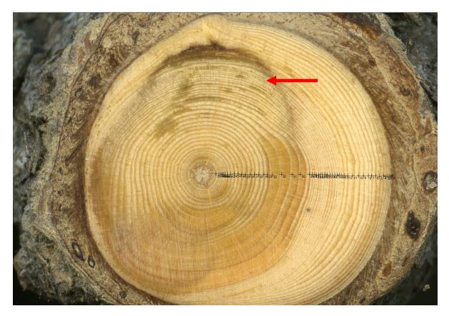
**Figure 5.** CooRecorder sample analysis (red arrow indicating the trample scar and the black markers showing successive tree ring dating).
