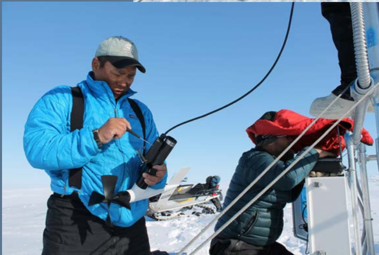
Installing weather stations for the Silalirijit Project. Credit: Shari Gearheard
