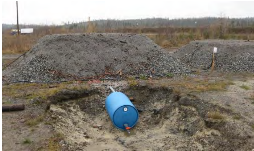
Figure 2. Barrel connected to base of Technosol lysimeter for collection of gravity through-flow water.
