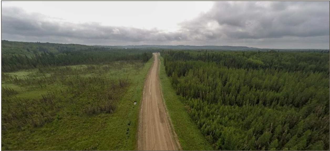
Figure 1. An example of a road acting as a barrier to water flow on a boreal wetland landscape. Note the ponding of water and dead trees on the left, with growth release on the right. Photo courtesy of Scott Nielsen (University of Alberta).
