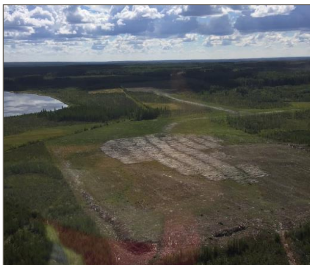
Figure 28. An example of road (left) and pad (right) construction at an in-situ oil sands facility using corduroy as a base foundation.
