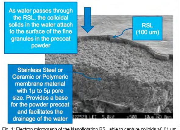
Fig. 1: Electron micrograph of the Nanoflotation RSL able to capture colloids >0.01  $\mu$ m in size on a stainless steel membrane with a pore size of 1  $\mu$ m.
