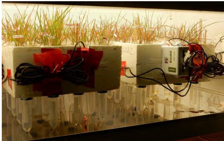
Figure 3. Soil Moisture Monitoring Probes and leachate sampling tubes connected to Styrofoam blocks.
