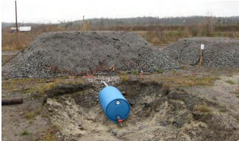
Figure 2. Barrel connected to base of Technosol lysimeter for collection of gravity through-flow water.
