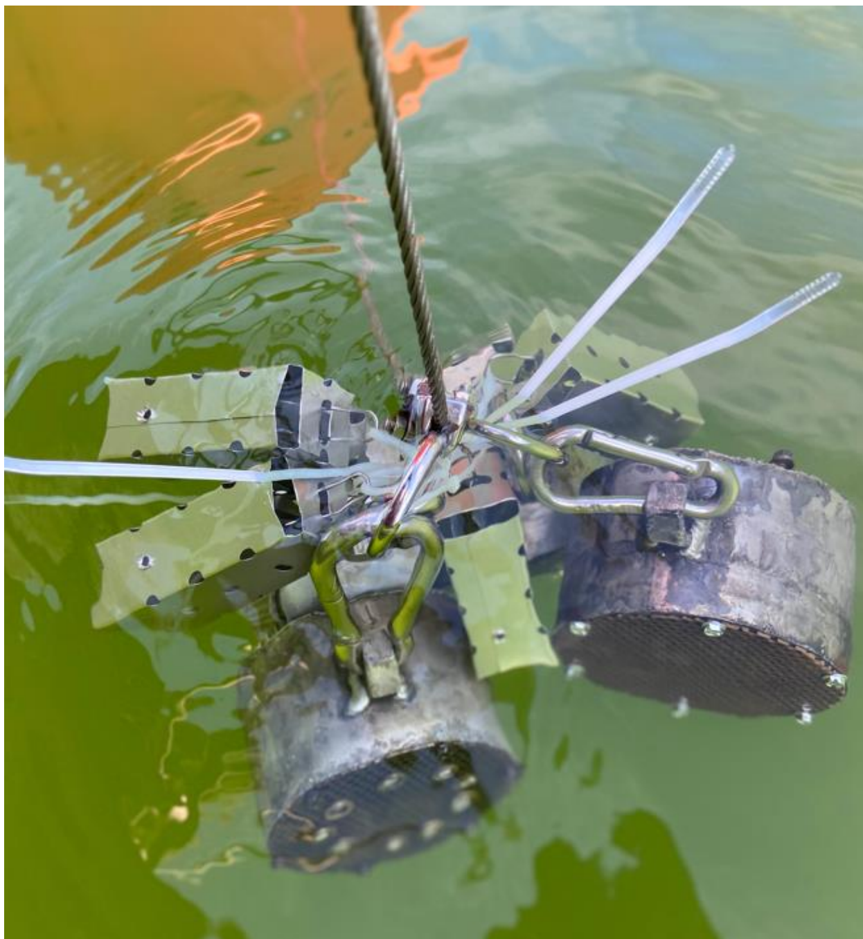
Figure 4. Deploying a polyethylene membrane device (PMD) into the water for 15-30 days during the summer. PMDs absorb polycyclic aromatic compounds (PACs) over time. Polycyclic aromatic hydrocarbons (PAHs) are at such low levels that they would be undetectable using regular water sampling methods.
